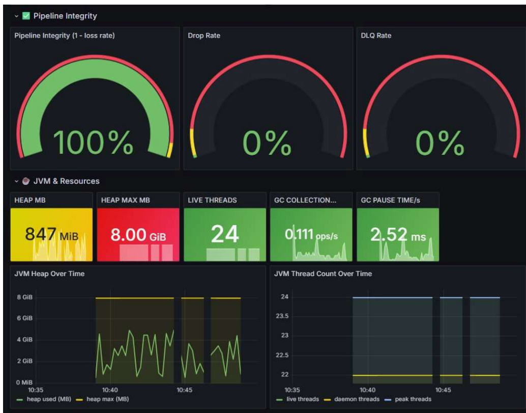
Image 3 — Integrity: 100%. Drop: 0%. DLQ: 0%. Heap: 847MB at snapshot, max 8GB. GC collection: 0.111 ops/s. GC pause: 2.52ms. 24 live threads stable.
