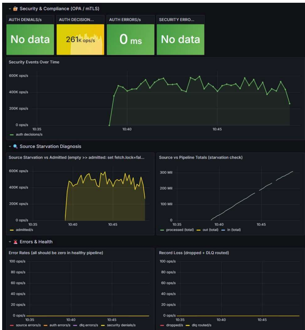
Image 2 — Auth decisions at 261K/sec tracking throughput. Zero errors across all categories. Zero record loss. Zero DLQ routes. Source starvation: none detected.
