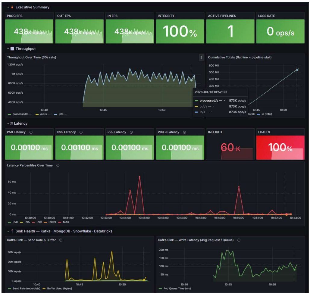
Image 1 — Executive: 438K ops/s at snapshot (873K at 10:52:30 tooltip). 100% integrity, 0 loss. P50/P95/P99/P99.9: all 0.001ms. Load: 100%. Kafka sink burst reaching 30M ops/s.
