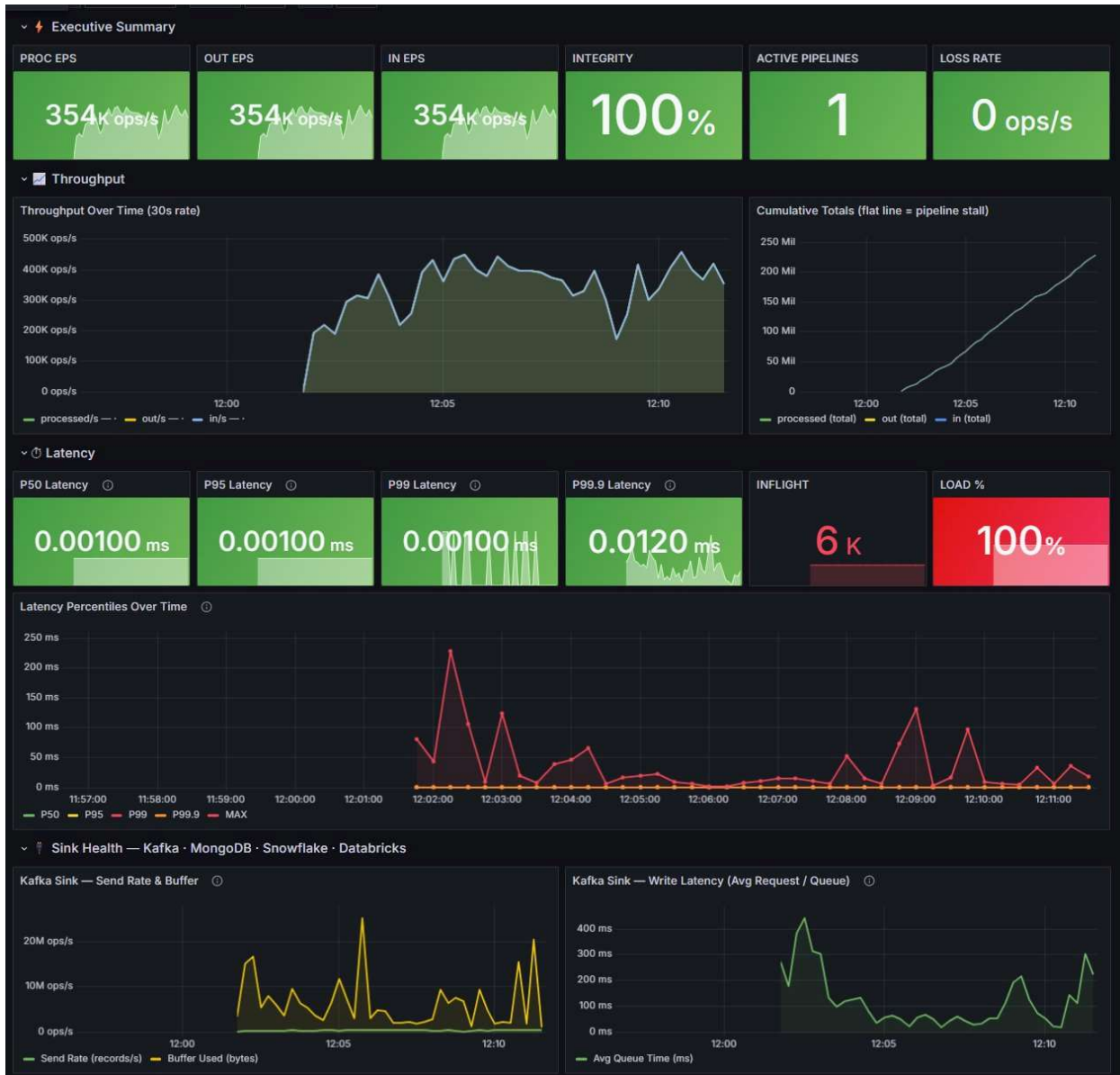
Image 4 — Executive summary: 354K ops/sec, 100% integrity, 1 active pipeline, 0 loss rate. P50/P95/P99 latency: sub-millisecond. P99.9 latency: 0.012ms. Kafka sink send rate reaching 20M+ ops/s burst. Load pinned at 100% — the machine is working.
