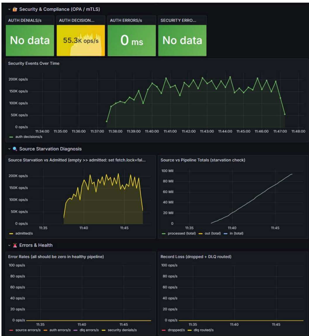
Image 3 — Auth decisions: 55.3K/sec. Zero denials, zero errors. Source vs Pipeline Totals: single overlapping line through 95M. Error rates and record loss: flat zero throughout.
