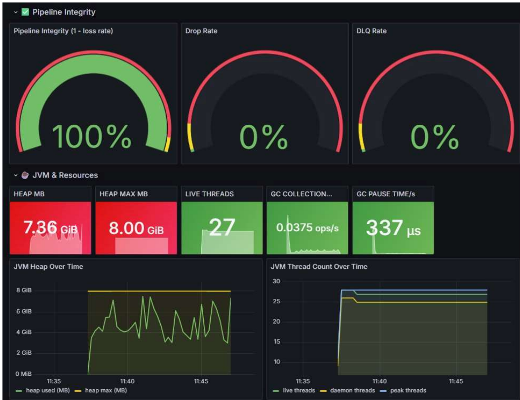
Image 4 — Integrity: 100%. Drop: 0%. DLQ: 0%. Heap: 7.36GiB at snapshot, max 8GiB. GC: 0.0375 ops/s, 337μs (Grafana 30s rate). GC log: 91 pauses, 23.1ms avg, 89.0ms max. Zero Full GC. 27 threads.
