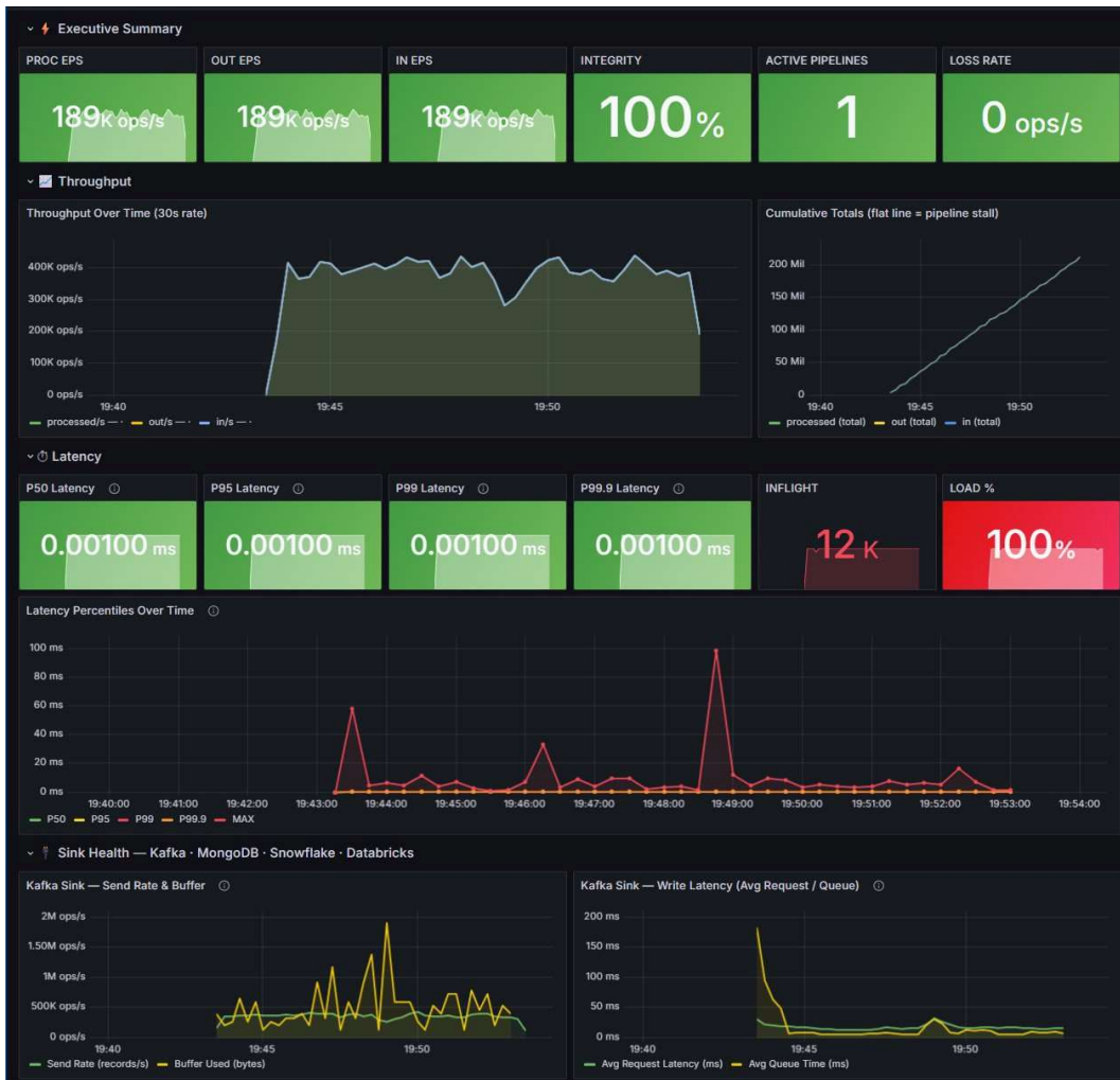
Image 1 — Executive: 189K ops/s snapshot (30s rate). Throughput chart: 300K–420K sustained plateau. P50/P95/P99/P99.9: all 0.001ms. INFLIGHT 12K. Kafka Sink: TLSv1.3 mTLS active, write latency near-zero after handshake.
