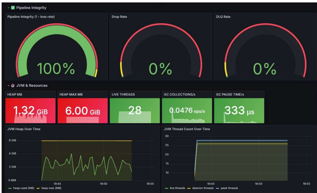
Image 2 — Integrity: 100%. Drop: 0%. DLQ: 0%. Heap: 1.32GiB at snapshot, max 6GiB. GC: 0.0476 ops/s, 333µs (Grafana 30s rate). GC log: 142 pauses, 14.0ms avg, 94.2ms max. Zero Full GC. 28 threads.
